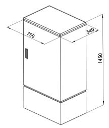
Standard capacity up to 576 cores, in three Models: GXF-144 (Dimensions: 1030\*570\*308), GXF-288 (Dimensions: 1450\*750\*320) and GXF-576 (Dimensions: 1450\*750\*540).
